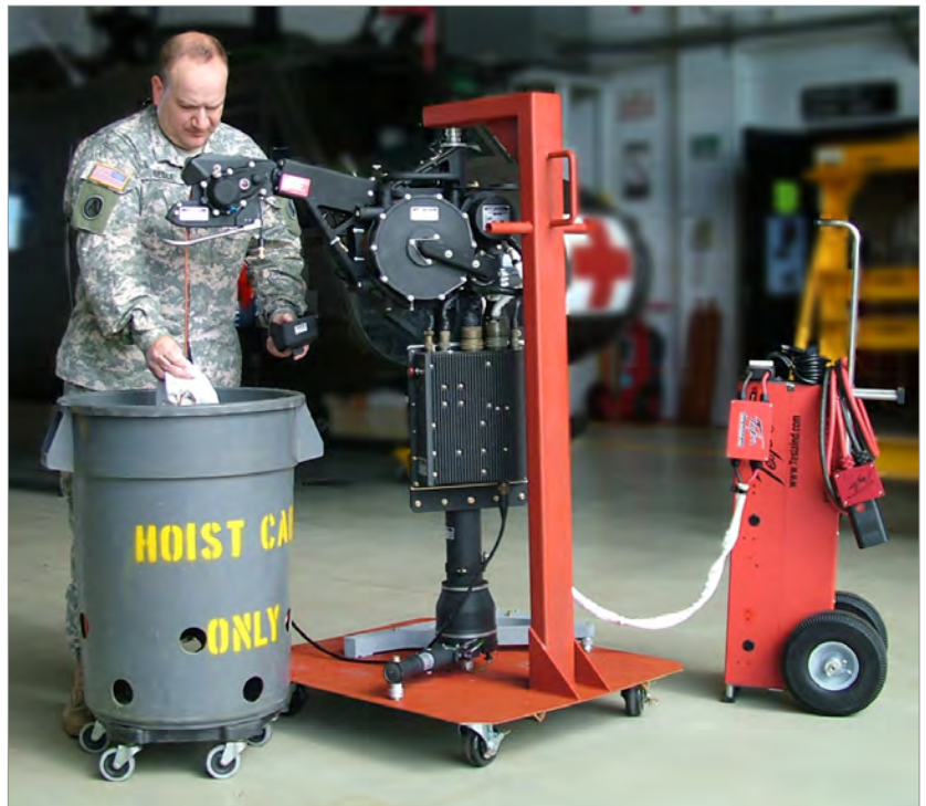
Figure 7: The TI2006-308 DC Universal Hoist Control Cable is designed to withstand daily military testing.
