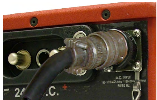
Figure 4.2.2 AC Input Line Cord Attached
