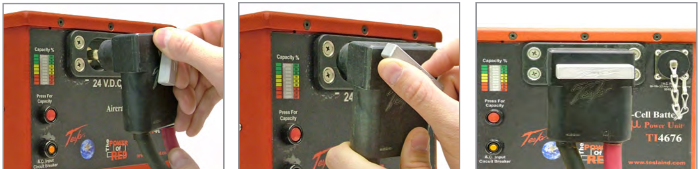
Figure 4.5.1 Attaching DC Power Cable to TI4676 MPU
