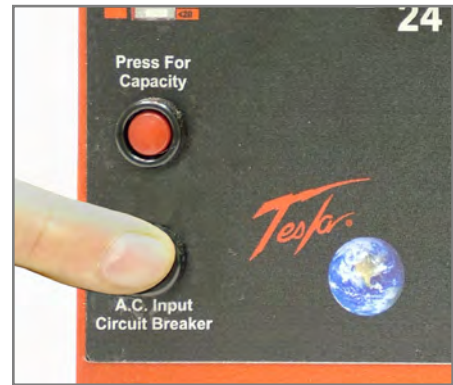
Figure 4.1.2 Pushing AC Input Circuit Breaker
