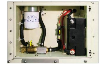
Figure 11: Oil Filter and Battery
