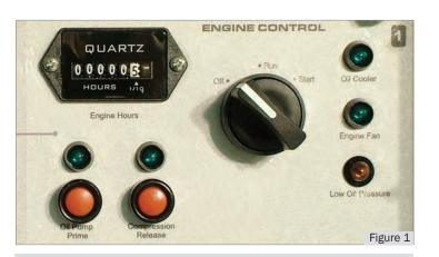
Figure 1: Engine Control Panel - Starter and Indicator LEDs
