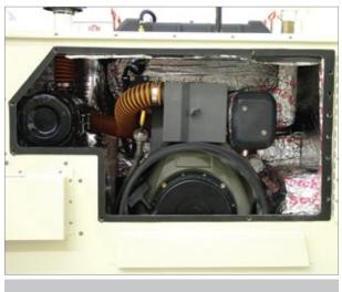
Right Engine Access Panel - Oil Dipstick, Air Filter, Pull Start
