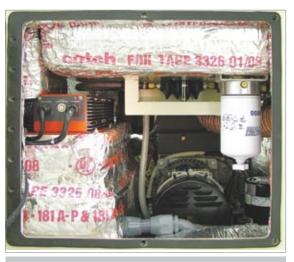
Left Engine Access Panel - Fuel Filter, Generator, Oil Cooler, and 2 internal Battery Chargers
