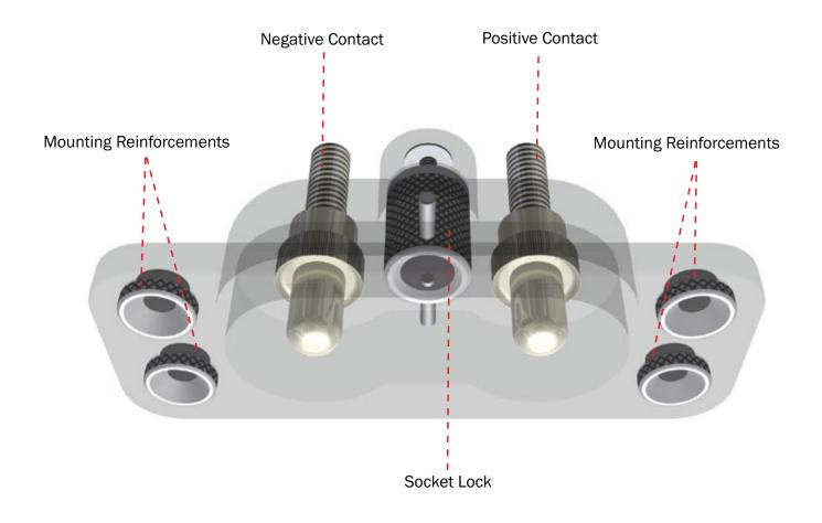
Attaching a dc plug to the Tesla<sup>™</sup> DC Battery Receptacle is quick and easy. **Step1:** line up the plug with the receptacle. **Step 2:** push forward while rotating the T-handle one full turn clockwise. **Step 3:** The unit is now ready to safely transfer 1500 A.
