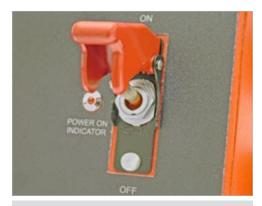
Figure 1: Power ON/OFF Switch and Indicator
