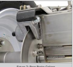
Figure 2: Rear Brake Caliper
